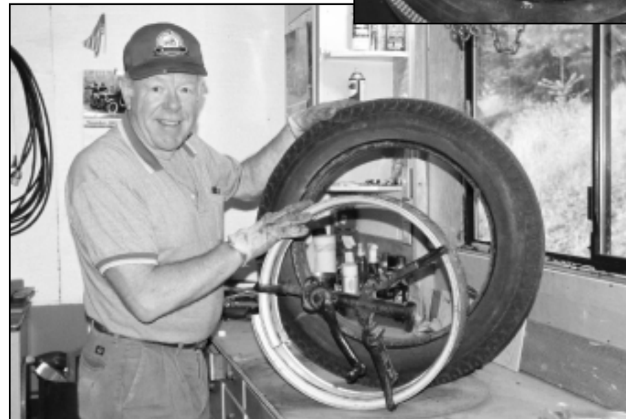
Alan Tiffany demonstrates the use of three-legged rim tool for spoke wheels.
